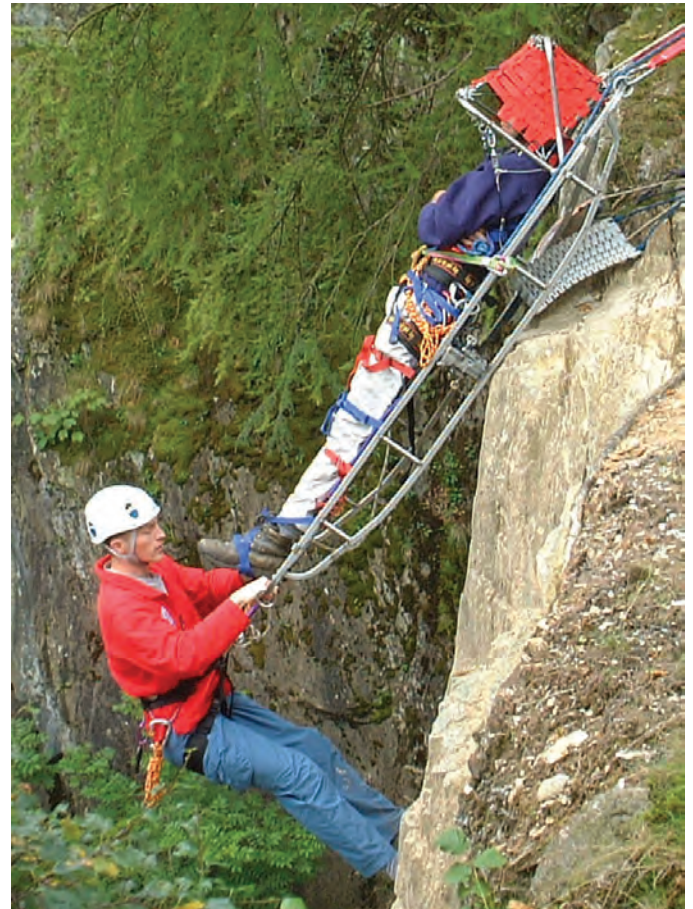
The stretcher becomes extremely vulnerable when subjected to a cantilever load
