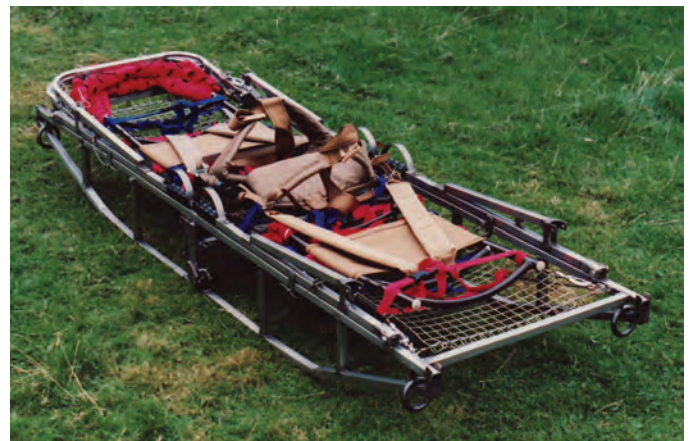
The Mark 3 Bell stretchers all had integral lift rings
