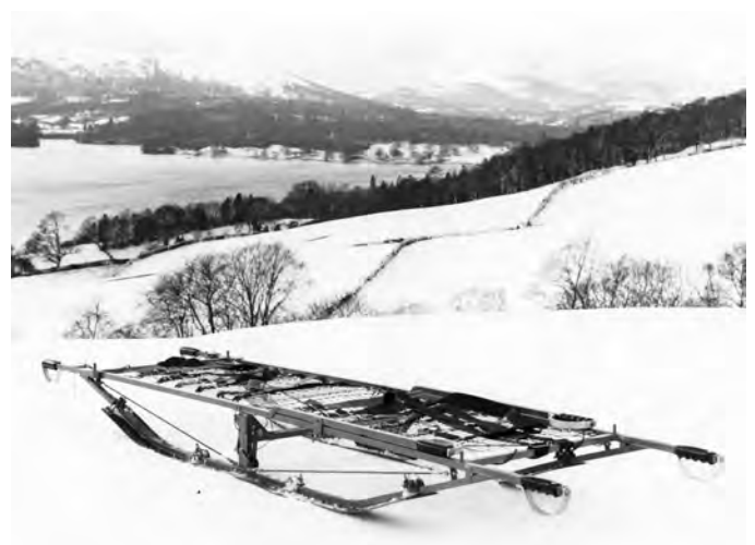
This late Mark 1 has modified handles for use with RAF Wessex helicopters
